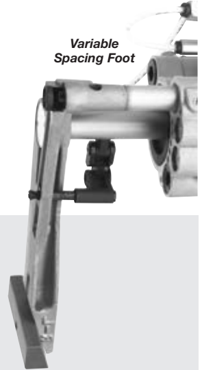
4. Depress the trigger. Immediately, the Mandrel is drawn back and the Collet locks the tool to the work. Simultaneously, the motor starts and the tool feeds forward to a positive stop. The tool then retracts automatically and returns to its starting position.
